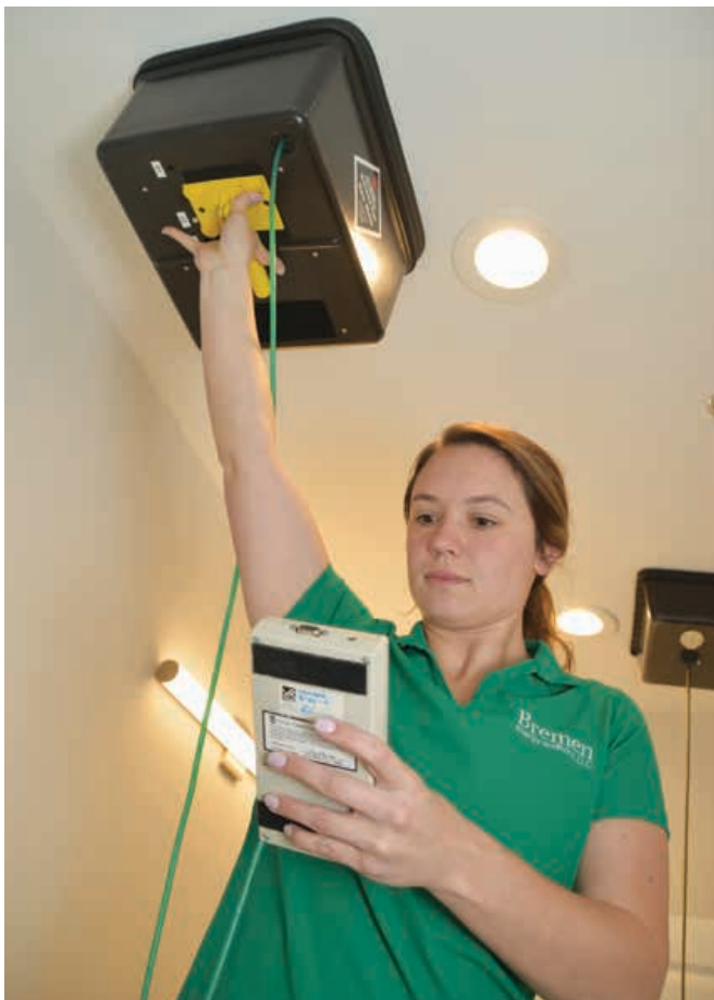
Clockwise from top, the W at Brannon Crossing apartment complex, Nicholasville. HERS Rater Field Inspector Abby Eipert performs a blower door test which measures air leakage. Field Technician Sydney Vaughn tests a bath fan to measure air quality. Photos: Rachel Settles
