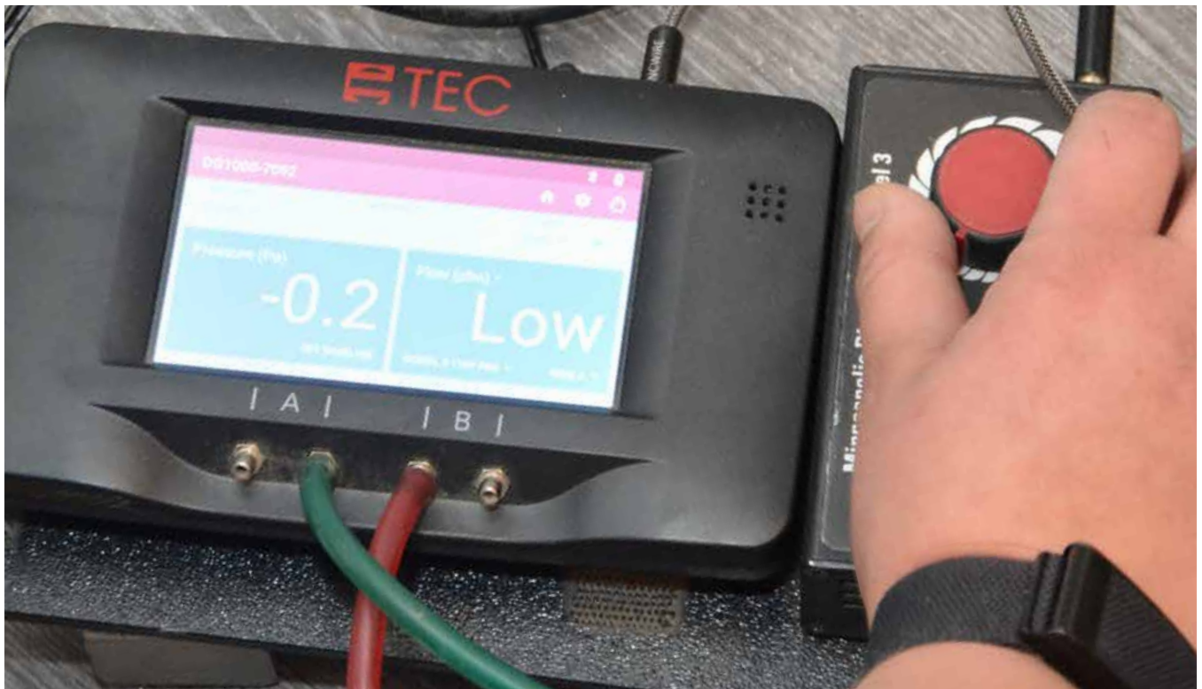
HERS Rater Field Inspector Abby Eipert tests duct leakage in an apartment at the W in Brannon Crossing, Nicholasville. Duct leakage is a leading cause of high bills. Photo: Rachel Settles
